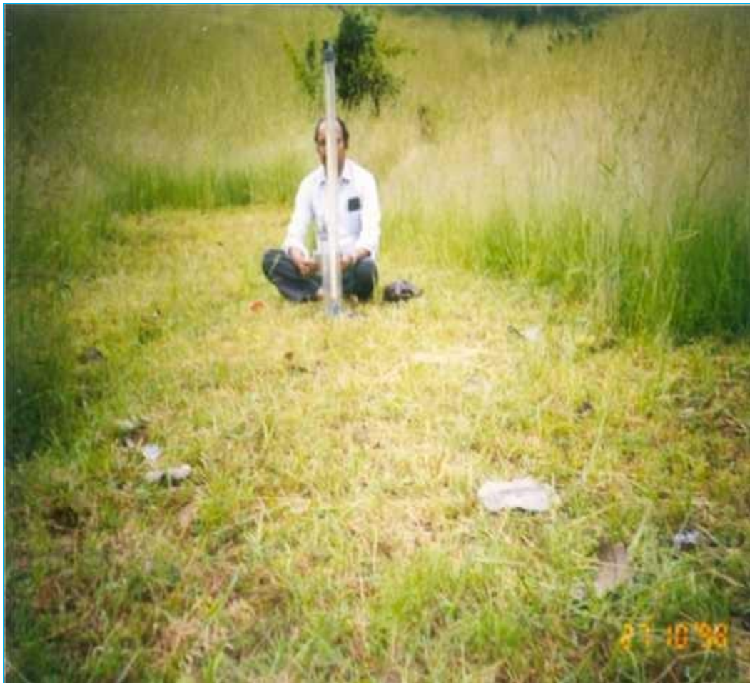
Figure 4.1 Disc Permeameter experiment to measure the soil hydraulic properties
